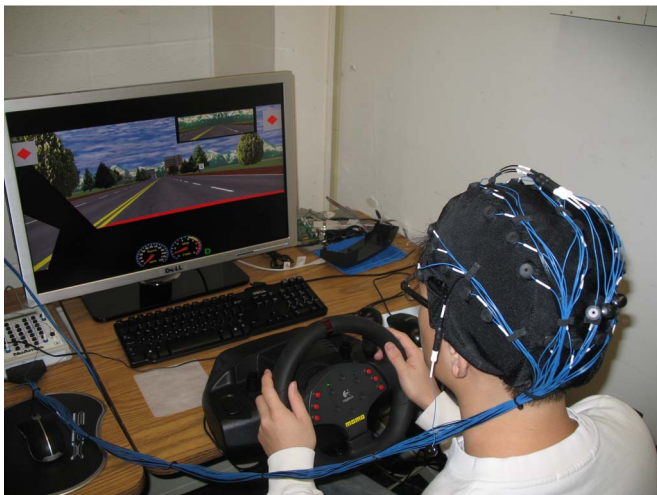
Fig. 1. Experiment setup using a STISIM driving simulator and a Neuroscan system including one Quik-Cap, Nuamps Express, and Scan software to record and analyze EEG signals during driving (the map for navigation is not included in this picture).
