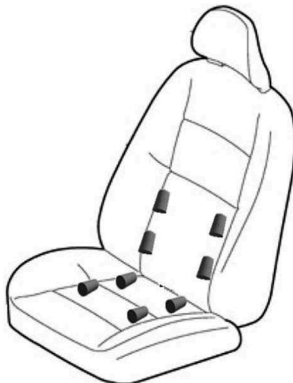
Figure 2. Haptic seat and the locations of the vibration motors used in the experiment.
